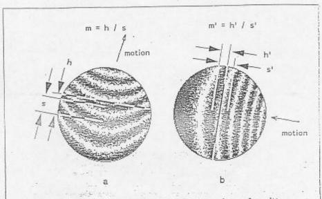
Figure A2.3 r Example showing 0,4 fringe spacings of sagitta error and 1,8 fringe spacings of irregularity, with the reference surface oriented in two directions (Evaluation in subclause A2.2.2).
