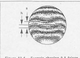
Figure A2.6 Example showing 0,5 fringe spacings of rotationally symmetric irregularity
