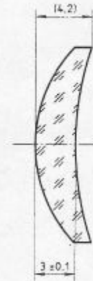
Figure 17 — Thickness indications for a meniscus lens element
