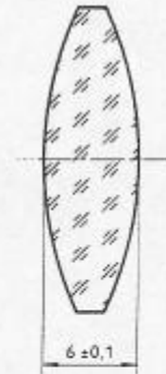
Figure 16 — Thickness indication for a biconvex lens element
