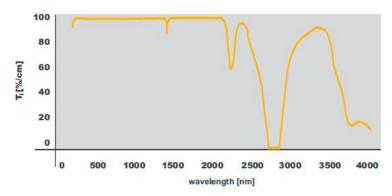
HPFS<sup>®</sup> Standard Grade is certified to meet T external ≥ 80%/cm @185nm (T internal ≥ 88%/cm @185nm), when measured through a polished, uncoated sample.
