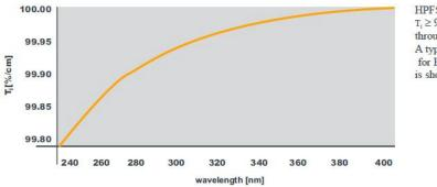
HPFS\* KrF Grade is certified to meet  $T_i \ge 99.8\%$ cm@248nm when measured through a polished, uncoated sample. A typical internal transmittance curve for HPFS\* KrF Grade fused silica is shown here.
